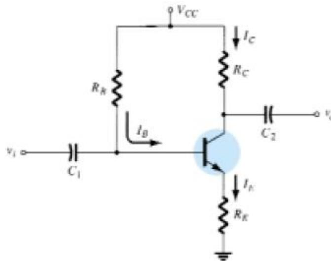
Fig.10: BJT bias circuit with emitter resistor.
