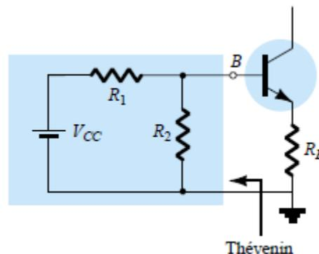
Fig.18: Redrawing the input side of the network of Fig. 16.
