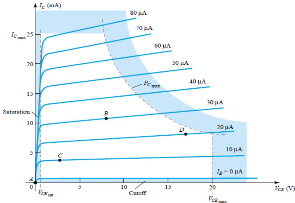
Fig.1: Various operating points within the limits of operation of a transistor
