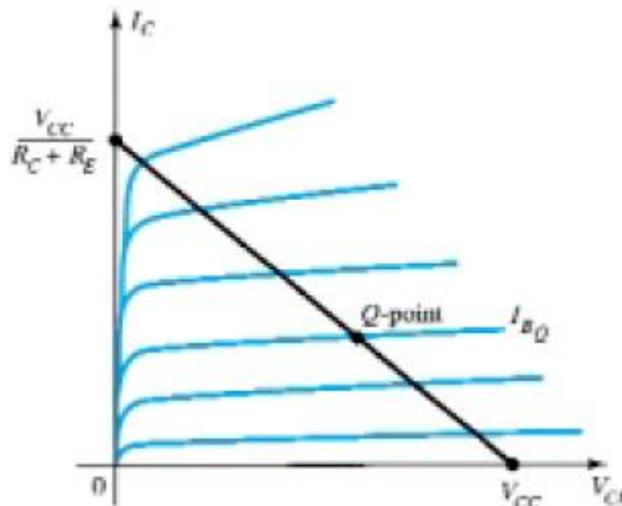
Fig. 15: Load line for the emitter-bias configuration
