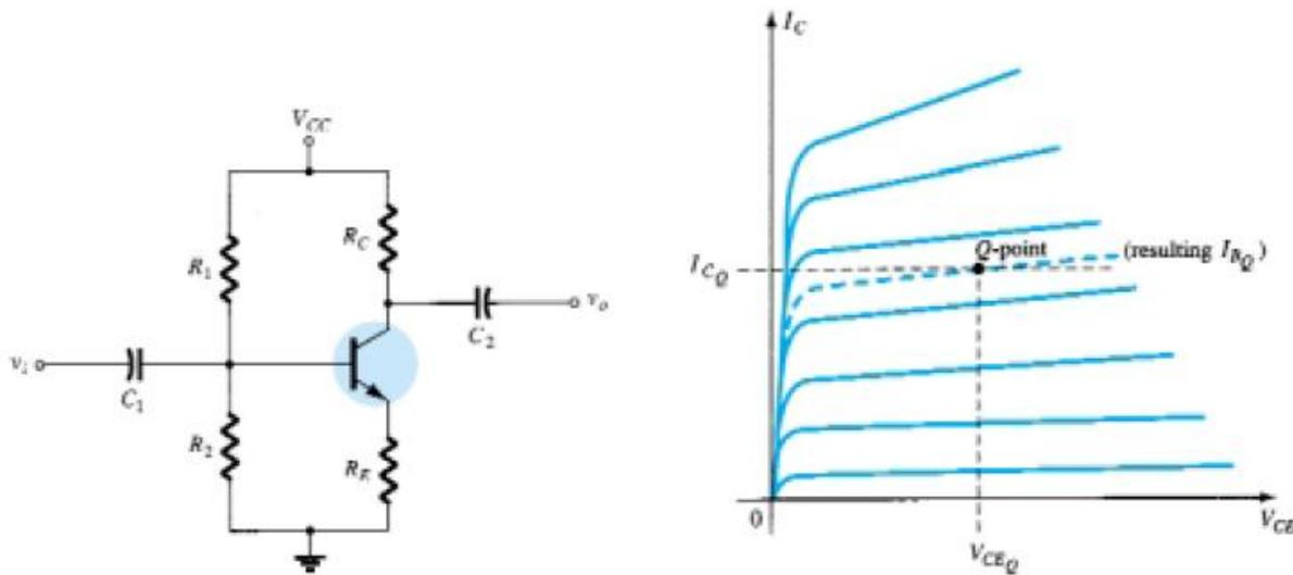
Fig.16: Voltage-divider bias configuration. Fig. 17: Defining the  $Q$ -point for the voltage-divider bias configuration.
