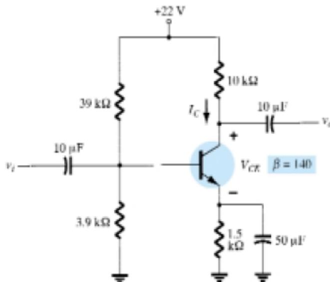
Fig.20: Beta-stabilized circuit for Example 4.7.
