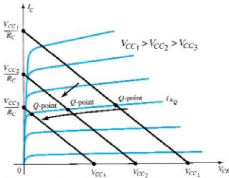
Fig.8: Effect of lower values of  $V_{CC}$  on the load line and  $Q$ -point
