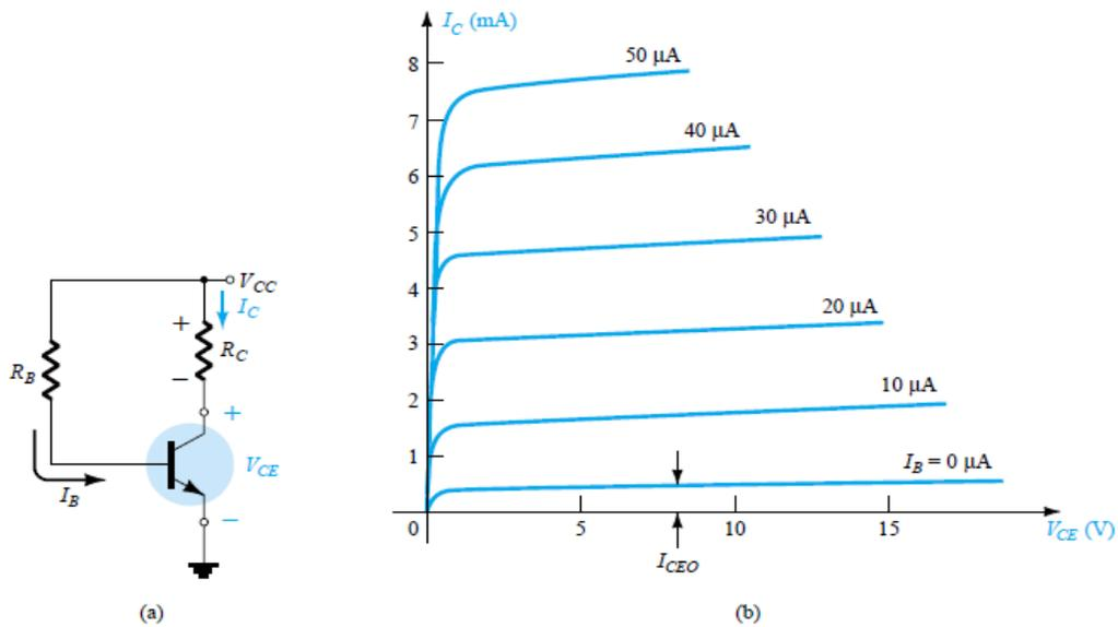
Fig.4: Load-line analysis: (a) the network; (b) the device characteristics.
