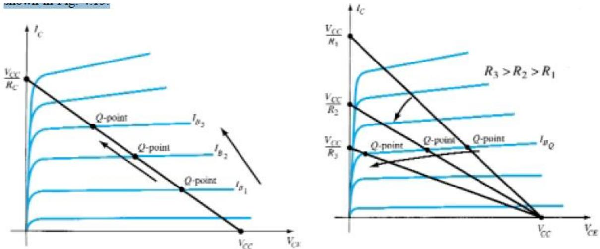
Fig.6 Movement of  $Q$ -point with increasing levels of  $I_B$ . Fig.7 Effect of increasing levels of  $R_C$  on the load line and  $Q$ -point
